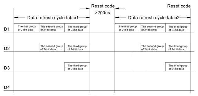
Note: the D1 sends data for MCU, D2, D3, D4 for data forwarding automatic shaping cascade circuit.
