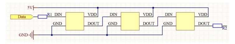
In the practical application circuit, the signal input and output pins of the IC signal input and output pins should be connected to the signal input and output terminals. In addition, in order to make the IC chip is more stable, even the capacitance between beads is essential back.
