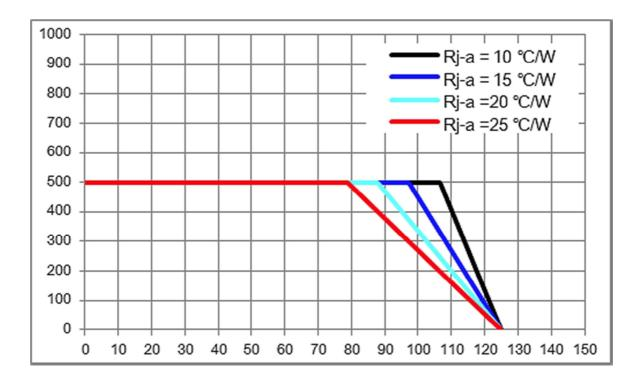
The junction temperature can be correlated to the thermal resistance between the junction and ambient (Rja) by the following equation.
