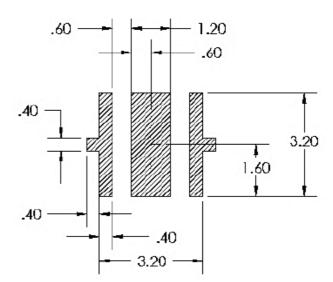
Recommended PCB Solder PAD (Suggest Stencil t=0.12 mm)
