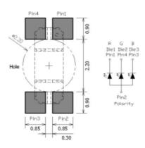
Figure 1. IN-S124TCR Solder Pattern
