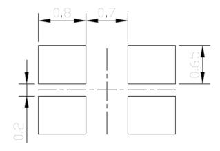
Figure 1. IN-S66TCTRGBE Solder Pattern
