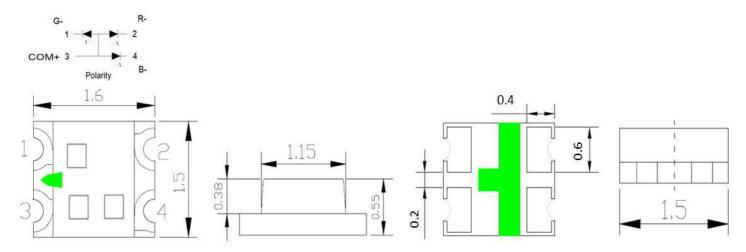
Figure 2. IN-S66TCTRGBE Package Dimensions
