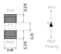
Figure 1. IN-S21AT5UW Solder Pattern
