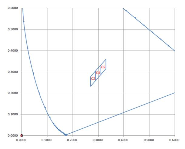
@5mA / Ta=25°C, It maintains a tolerance of x,y  $\pm$  0.007
