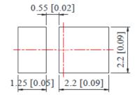
Figure 1. IN-P23CTKG Solder Pattern
