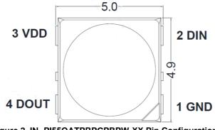
Figure 2. IN- PI55QATPRPGPBPW-XX Pin Configuration
