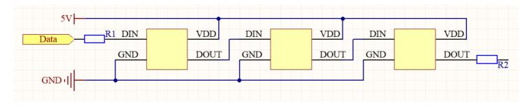
Product signal input and output must be connected in series with protection resistor R1. R1 depends on the size of the cascade amount, the greater the number of cascade, the smaller R1. The general recommended value is between  $200-2K\Omega$ , usually the recommended value is typical  $500\Omega$ .
