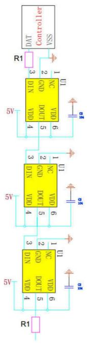
In the practical application circuit, the signal input and output pins of the IC signal input and output pins should be connected to the signal input and output terminals. In addition, to make the IC chip is more stable, even the capacitance between beads is essential back.
