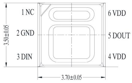
Figure 2. IN- PI35QBTPRPGPBPW-XX Pin Configuration
