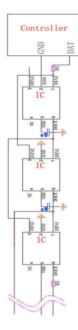
Product signal input and output must be connected in series with protection resistor R1. R1 depends on the size of the cascade amount, the greater the number of cascades, the smaller R1. The general recommended value is between  $200-2K\Omega$ , usually the recommended value is typical  $500\Omega$ .
