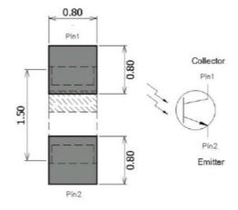
Figure 1. IN-S63CTLS Solder Pattern
