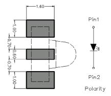
Figure 1. IN-S126ESGHIR Solder Pattern
