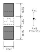
Figure 1. IN-S42CTQIR Solder Pattern
